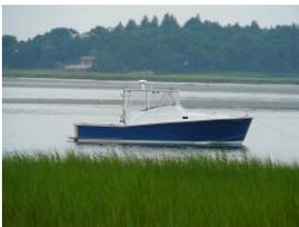
**ATLANTIC** is a custom, cold molded sport fishing design modified for cruising. Designed by Eldridge McInnis, the hull is a modified Fortier 33 with a higher deck and custom sheer, allowing for greater interior volume, increased deck area, and an extremely dry ride.
